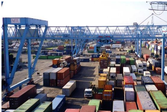
Rys. 8. Suwnica placowa (RailMounted Gantry crane – RMG)
