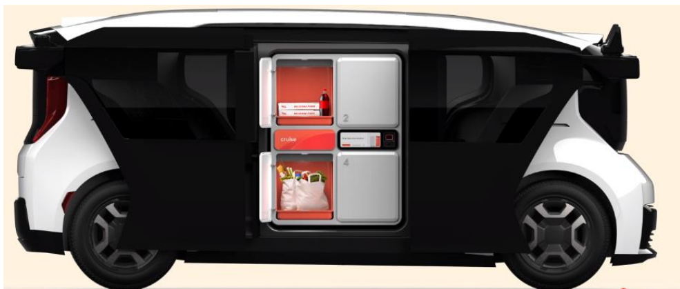
Fig. 5. Lockers of the origin model
